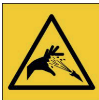
Figure 22. Hydraulic fluid under pressure
