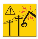
Always pay attention when working close to electrical cables. Maintain a safe distance. Bear in mind the risk of unforeseen movements. If the cutter should come into contact with a power line for any reason:
